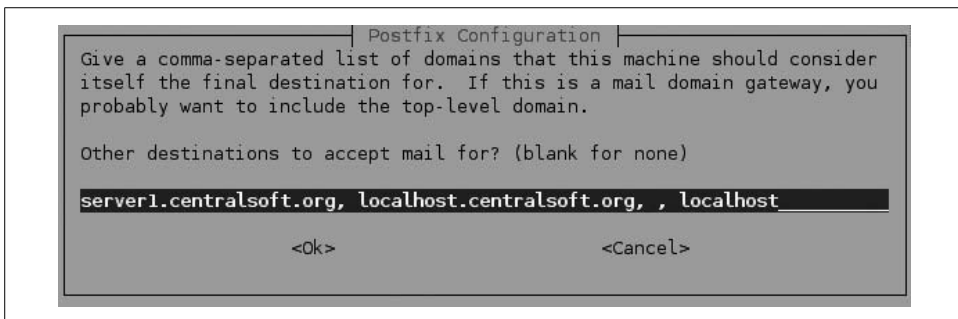
Figure 2-7. Internal domain list in used in Postfix
