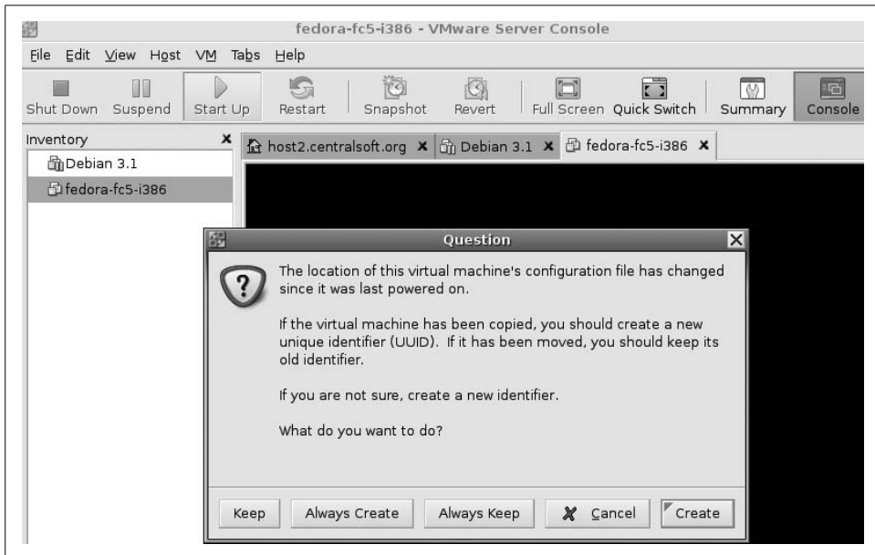
Figure 9-8. VMware asks about a virtual machine image's unique identifier
