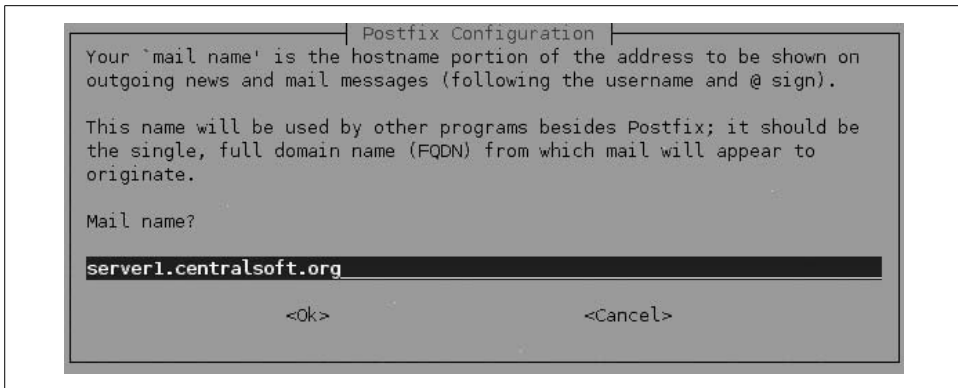
Figure 2-6. Checking the fully qualified domain name set for Postfix
