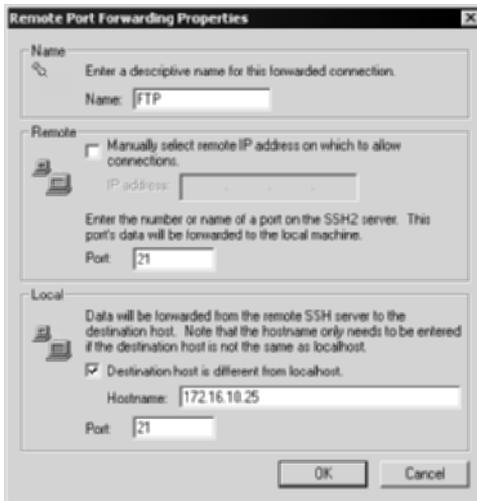
**Figure 6.9** Remote port-forwarding rules in an SSH client.
