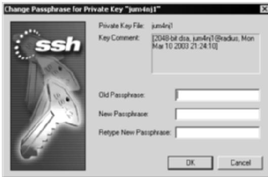
**Figure 4.10** The screen to change a passphrase with SSH Communications' GUI client.
