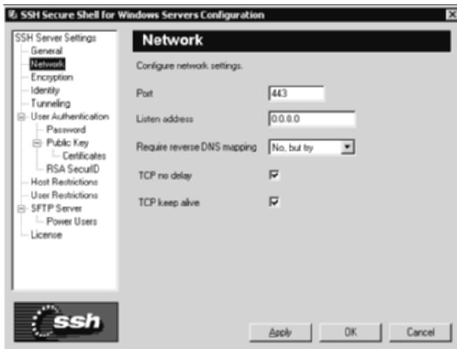
**Figure 2.3** Network screen from the SSH server configuration tool.
