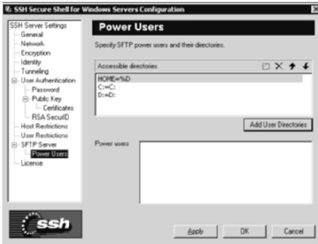
**Figure 2.13** SFTP Server–Power Users screen from the SSH server configuration tool.
