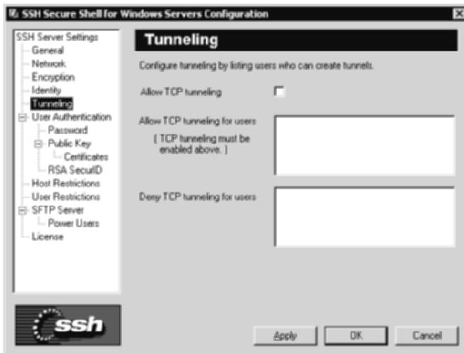
**Figure 2.9** Tunneling screen from the SSH server configuration tool.
