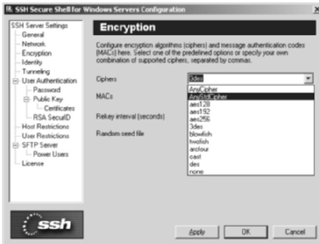
**Figure 10.13** Encryption section for SSH Communications' SSH server.
