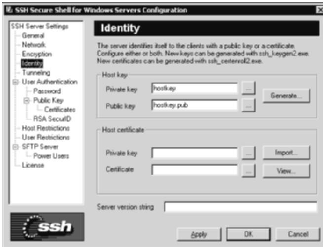
**Figure 2.8** Identity screen from the SSH server configuration tool.
