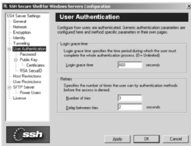
**Figure 4.1** The User Authentication section of the screen for SSH Communications' SSH server.
