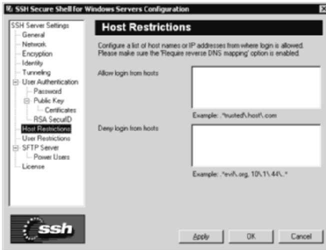
**Figure 2.10** Host Restrictions screen from the SSH server configuration tool.
