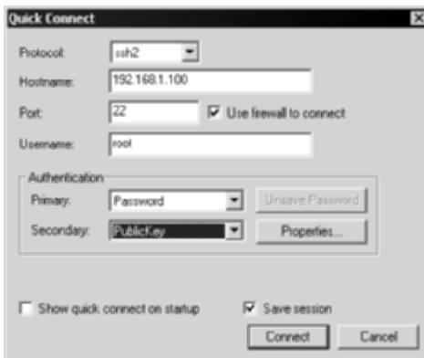
**Figure 5.7** SecureCRT client using SOCKS firewall setting.
