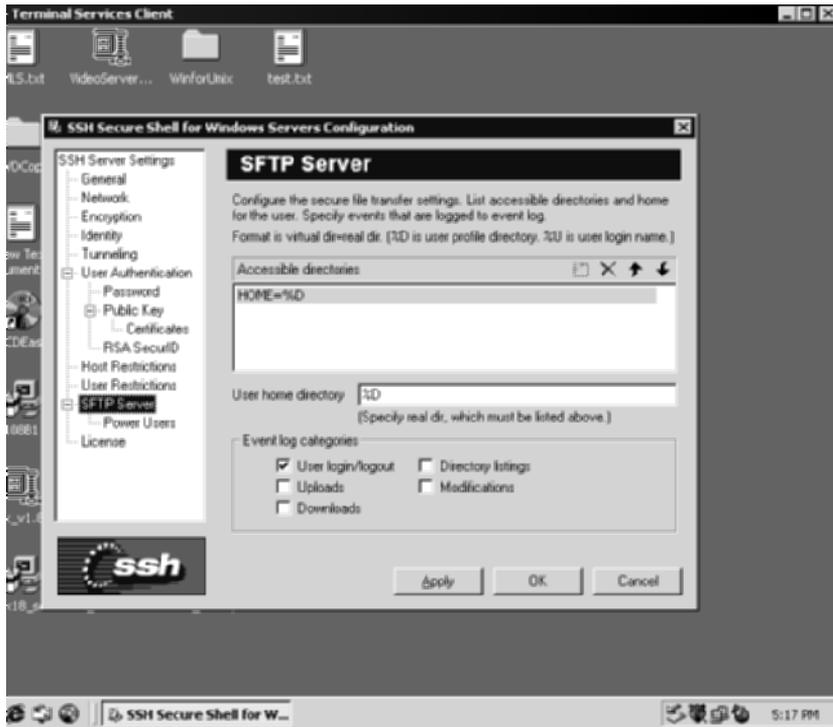
**Figure 2.12** SFTP Server screen from the SSH server configuration tool.
