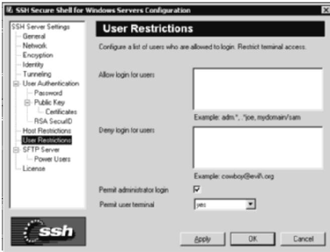
**Figure 2.11** User Restrictions screen from the SSH server configuration tool.
