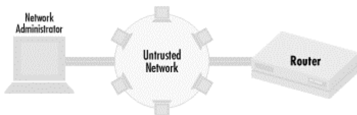
Figure 3.15. Managing a router through untrusted networks
