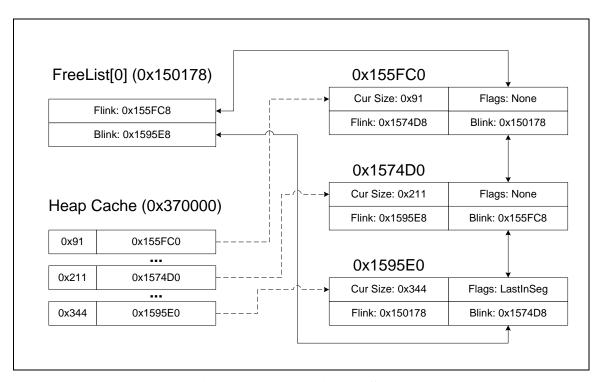
Figure 16 – Insert Attack Step 1
