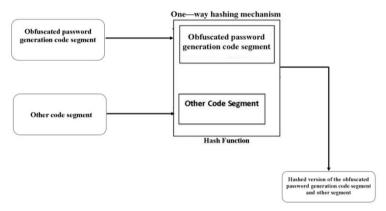
Fig. 2: Encryption (One - Way Hashing) Mechanism Module
