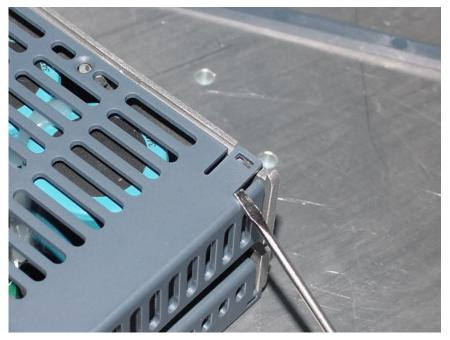
9. Once both locking tabs are seated, reinsert the single drive cover screw.
