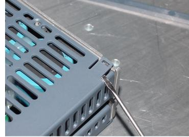
While lifting on the 1<sup>st</sup> tab, (as shown in #1) insert a larger, wide, flat screwdriver (shown below) between the drive cover and the last fin of the heatsink to separate and start the cover off to unlock the 1st tab.
