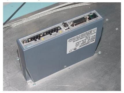
The DC model cover is held into place by a single (Philips) screw. Remove this screw in a static free area using wrist straps when coming in contact with the control board and its components.
