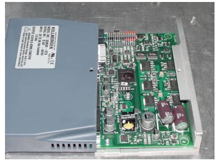
The EPROM /socket is now visible and accessible. Wear a static wristband when performing the following operations.
