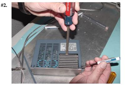
Carefully lift the remaining tab. The cover can be separated from the rear of the mounting heatsink as shown below/
