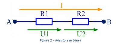
In case of serial connection (see Figure), the same current flows through the two resistors, so their current equals. This follows that the voltage of the resistor  $R_1$  is  $U_1 = R_1 \bullet I$  while the voltage of the resistor  $R_2$  is  $U_2 = R_2 \bullet I$  and  $U_1 + U_2 = U$ .
