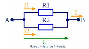
In case of parallel connection, the voltage of the resistors will be the same, since both of their terminals are connected. Then the current of the two resistors is  $I_1 = \frac{U}{R_1}$  and  $I_2 = \frac{U}{R_2}$ . The equivalent resistance in this case can be derived from Ohm's Law.
