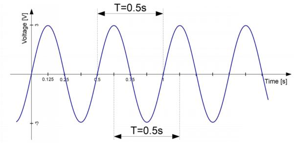
Figure 1 – Sinusoidal alternating voltage
