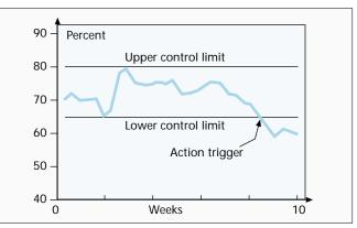
Figure 8. Early warning system: event trigger.
