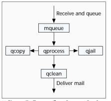
Figure 7. *Process flow diagram for the SMTP filter.*
