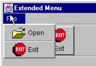
Figure 30.1 – A menu with pictures using the same Action object as the toolbuttons.
