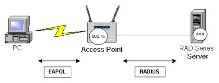
Figure 1 – A client authenticates by using EAPOL to communicate with the Access Point. The Access Point communicates with the AAA server using RADIUS.
