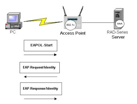
Figure 2 – The Start Phase. The supplicant (client) sends an EAPOL-Start message. The authenticator responds with an EAP-Request/Identity message. Finally, the supplicant responds with an EAP-Response/Identity message which contains the identity of the user.
