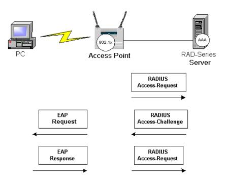
Figure 3 – The Authenticate Phase. The authenticator sends a RADIUS Access-Request message. The AAA server issues a challenge that is carried via EAP to the supplicant. The supplicant responds and the authenticator issues another RADIUS access request.
