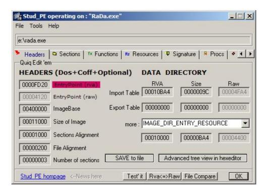
Figure 9: RaDa file PE header with StudPE
