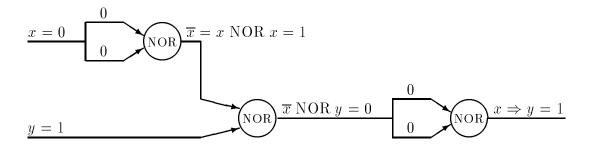
Figure 2.5: A NOR circuit computing  $x \Rightarrow y$ , with assignment on edges
