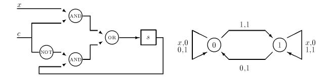
Figure 2.8: Circuit and state-transition diagram of a memory cell
